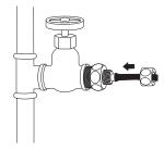
10. **Open** the auxiliary tap 1. **Open** the water supply shut-off valve to start water flowing through the system 2.
