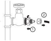
Push red hose over barb on hose nipple and tighten nut with a wrench. Ensure all connections are leak free.
